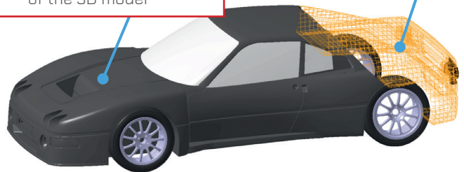
The result: Virtual 3D Model to use with AirShapers online Aerodynamic Analysis
